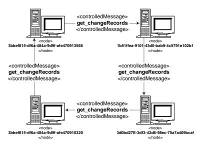
The communication graph described in the following example represents a spanning cycle topology. This is one of many possible topologies supported within this replication framework.
